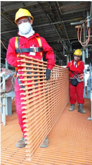
DURAGRID® Phenolic Grating's unique construction allows for many penetrations to be cut without adding additional supports.
